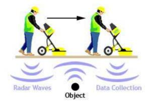
Figure 3: Working of a GPR.
