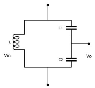
Figure 4: Capacitance Voltage Divider.
